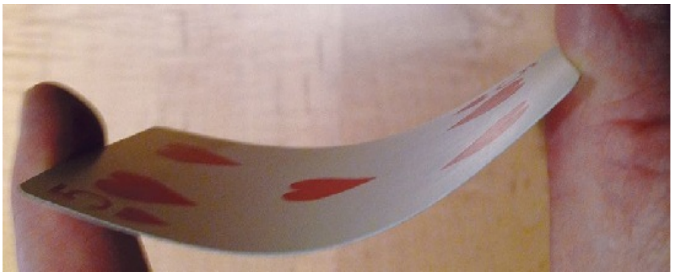
Fig. 23.8. A playing card, compressed end to end, bends and then buckles.
