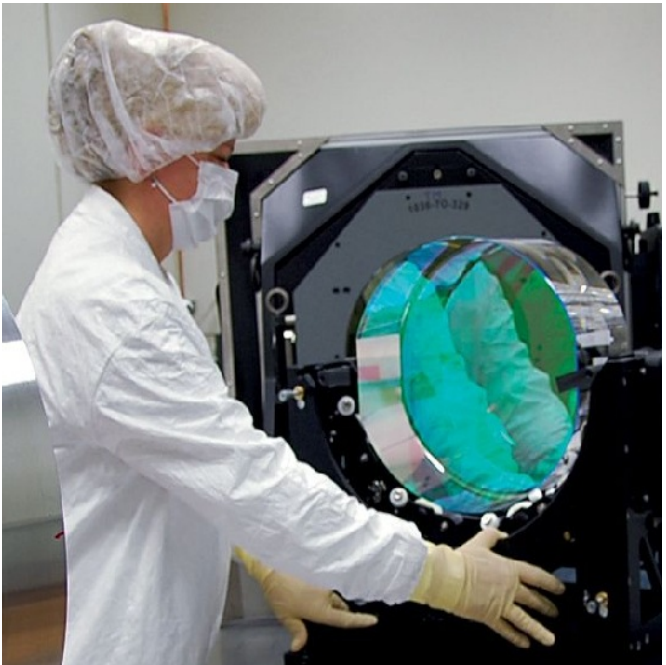
Fig. 26.2. A 40-kilogram mirror being prepared for installation in LIGO. Its location fluctuates, quantum mechanically, very, very slightly: one ten-billionth the diameter of an atom.
